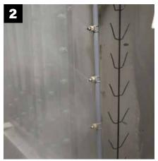
The product enters a heated cleaning stage to remove extrusion debris and fabrication oils.
