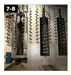
A 200 MPH air blast removes water drops from the pre-treated aluminum.
